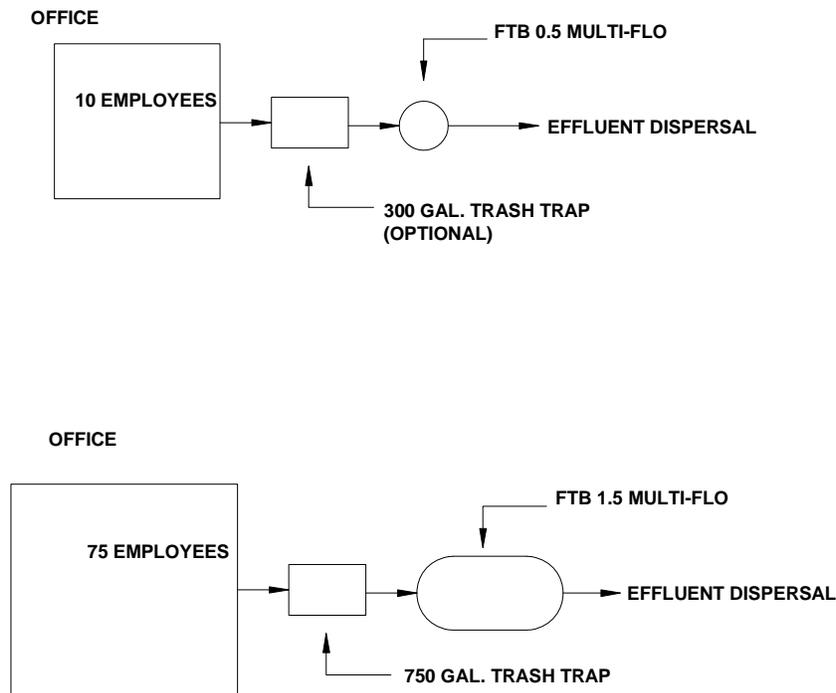
Figure 10—Commercial Occupancy Multi-Flo Installation with Flow Equalization
