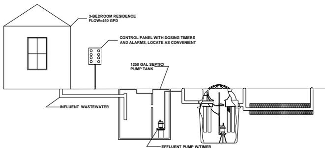
**Figure 9 - Multi-Flo Installation With Flow Equalization**
