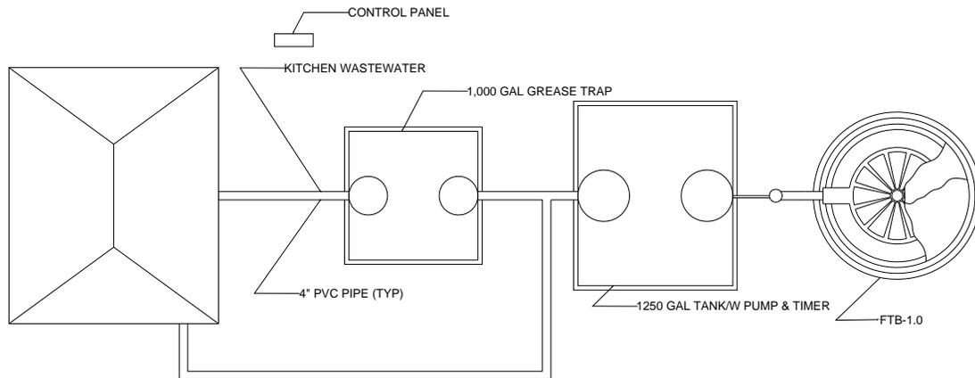
Figure 11—Plan View Showing Grease Trap
